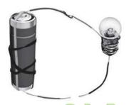
Circuit is open or broken. Therefore, bulb will not glow.
